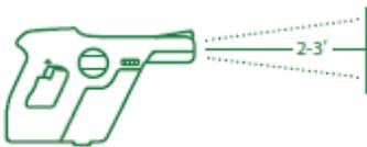
The optimum sprayer distance is 2-3 feet (0.6-0.9m) from the surface being sprayed.
