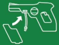
1. Align tank grooves into slide rail & lower sprayer unit onto the tank
